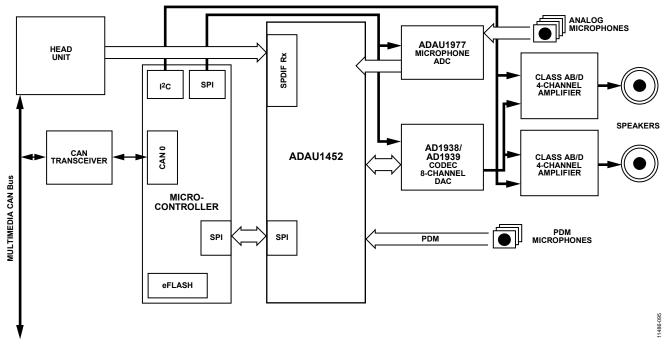
Figure 86. Automotive Infotainment Amplifier Block Diagram
