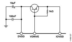
Figure 21. External Components Required for Voltage Regulator Circuit
