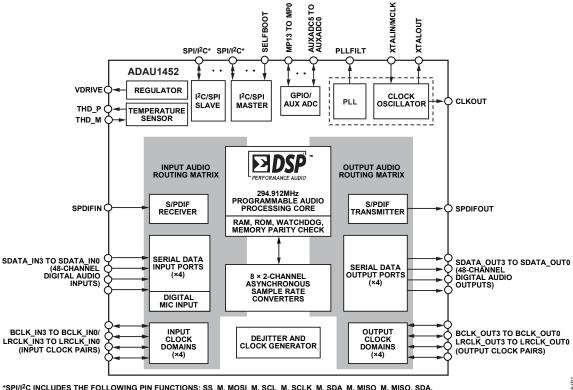
\*SPI/I<sup>2</sup>C INCLUDES THE FOLLOWING PIN FUNCTIONS: SS\_M, MOSI\_M, SCL\_M, SCLK\_M, SDA\_M, MISO\_M, MISO, SDA, SCLK, SCL, MOSI, ADDR1, SS, AND ADDR0 PINS.
