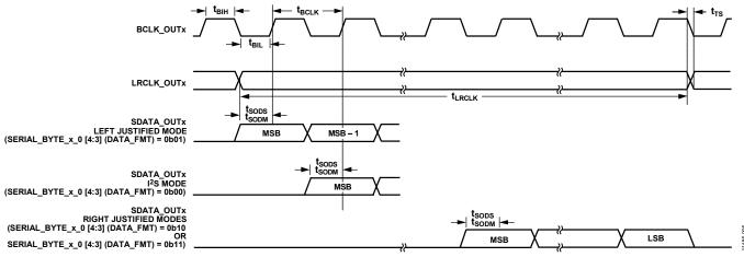
Figure 5. Serial Output Port Timing Specifications Rev. A | Page 8 of 176
