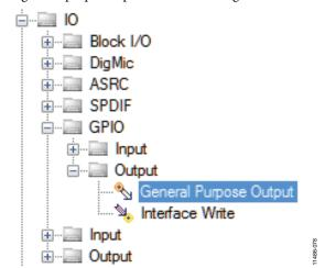
Figure 73. General-Purpose Output in the SigmaStudio Toolbox
