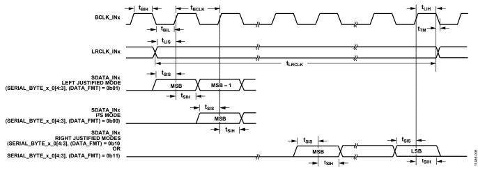
Figure 4. Serial Input Port Timing Specifications
