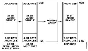
Figure 65. 32-Bit Serial Input Example
