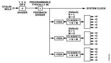
Figure 17. PLL and Clock Generators Block Diagram
