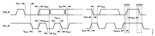
Figure 7. I<sup>2</sup>C Master Port Timing Specifications
