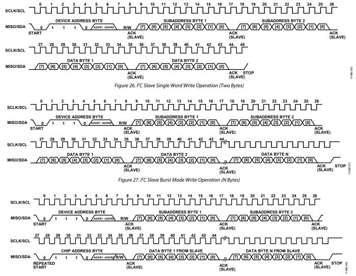
Figure 28. I<sup>2</sup>C Slave Burst Mode Read Operation (N Bytes)
