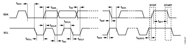
Figure 6. I<sup>2</sup>C Slave Port Timing Specifications
