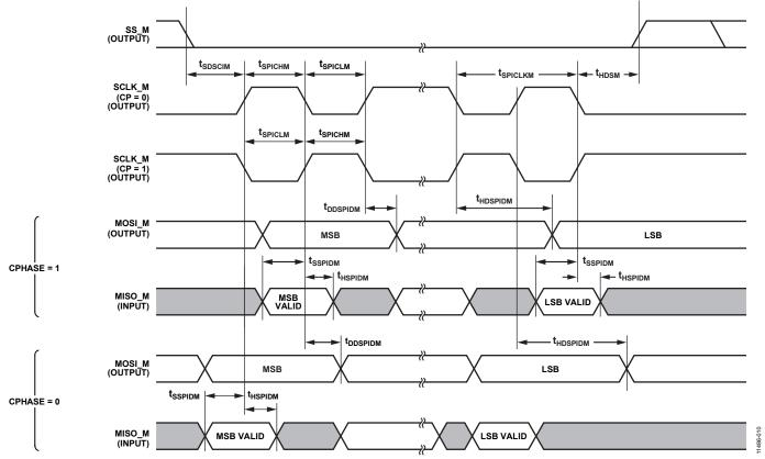
Figure 9. SPI Master Port Timing Specifications
