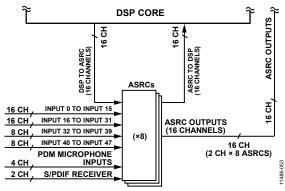
Figure 49. Channel Routing to ASRC Inputs
