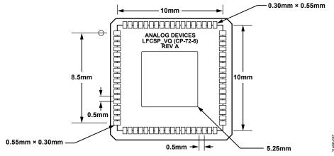
Figure 89. PCB Decal Dimensions
