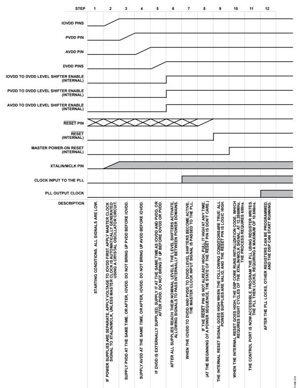
Figure 13. Power Sequencing and POR Timing Diagram for a System with Separate Power Supplies
