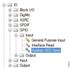
Figure 76. Auxiliary ADC Input Cell in the SigmaStudio Toolbox
