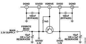
Figure 85. Ferrite Bead Power Supply Isolation Circuit Example
