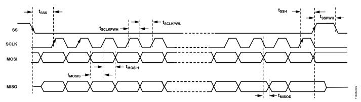
Figure 8. SPI Slave Port Timing Specifications
