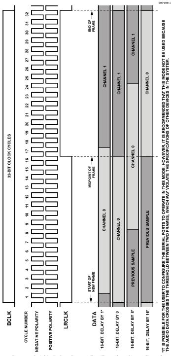
Figure 64. Serial Audio Data Formats; Two Channels, 16 Bits per Channel
