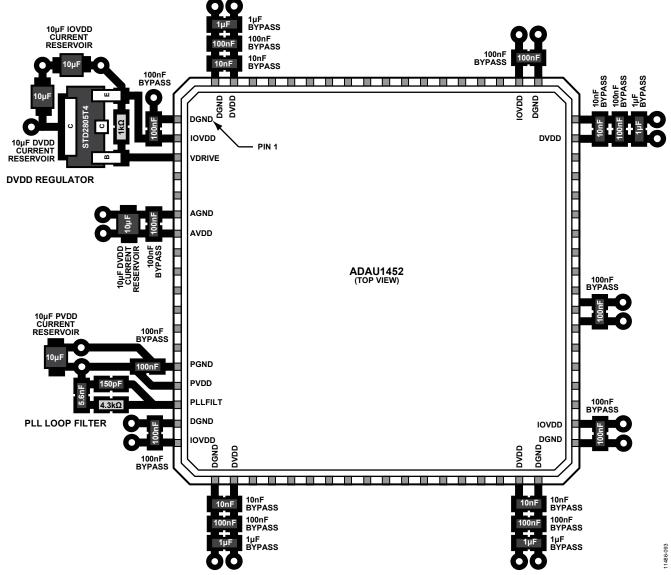
Figure 87. Supporting Component Placement and Layout
