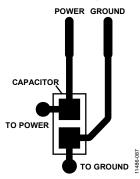
Figure 80. Recommended Power Supply Bypass Capacitor Layout
