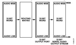
Figure 66. 32-Bit Serial Output Example
