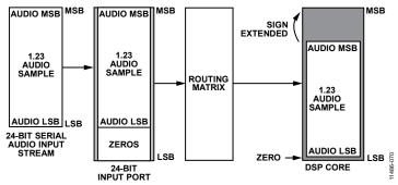
Figure 67. 24-Bit Serial Input Example
