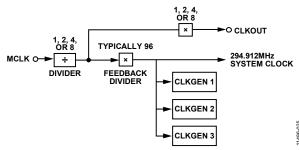
Figure 20. Clock Output Generator
