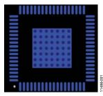
Figure 84. Exposed Pad Layout Example—Top View
