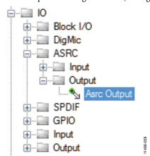
Figure 54. Location of DSP-to-ASRC Output Cell in SigmaStudio Toolbox
