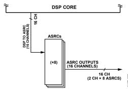
Figure 53. Example ASRC Routing for Asynchronous Serial Output from the DSP Care
