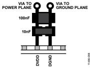
Figure 81. Layout for Multiple Power Supply Bypass Capacitors
