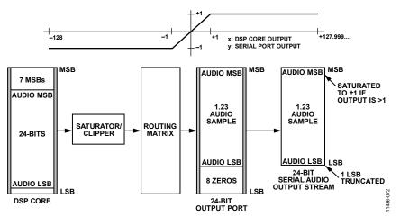
Figure 68. 24-Bit Serial Output Example
